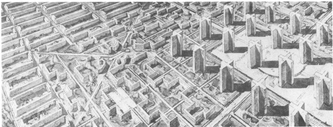
Figure 2. Three building types in the Ville Contemporaine , 1922: on the right, sixty-storey office towers; centre twelve-storey 'setback' residential blocks; left residential blocks on the 'cellular' principle. (Source: City of Tomorrow , p.169)
